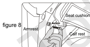
Figure: hex head screw fixed in front part of armrest
